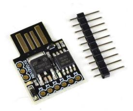
The ATtiny85 is a low-power, high-performance 8-bit microcontroller with 8 KB of flash memory and 512 bytes of SRAM. The module is ideal for small and compact projects, such as wearable electronics, where space and power consumption are critical factors. The board is commonly used for DIY electronics projects, hobbyist inventions, and educational purposes.
