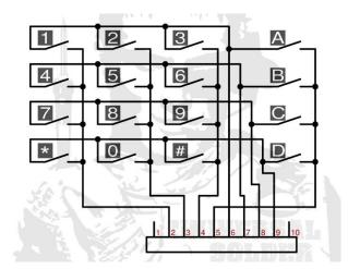
A keypad in 4 x 4 matrix configuration and conveniently small size of 65 x 68mm.
