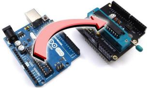
2. Attach the Programming Shield to your Arduino UNO.
