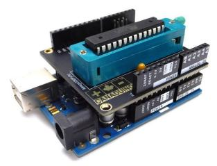
1. Remove the ATmega328P-PU from your Arduino UNO and install it on the Programming Shield.
