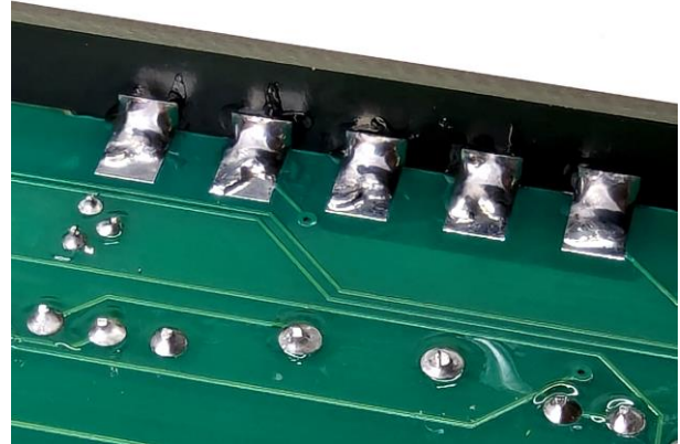
Solder blobs for contact and stability
