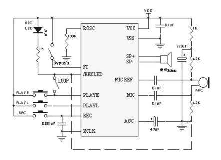
Picture shows a general example of a circuit with the ISD1820, not the actual module.
